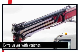
A well-known and usual hose routing to the end of the extensions means that 1 or 2 extra valves are fed in sturdy hose guides alongside the jib extension system. If further efficient protection of the hoses is required, 1 or 2 extra valves can be fed in internal hose reels and lie particularly well protected.
